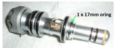
3. Slide Eigenbolt spacer onto the bolt guide, locking the interior o-ring or internal rib into the bumper groove in the rearmost position. You should feel the spacer click into place.
