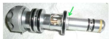
2. Remove bumper o-ring at the base of the bolt guide.
